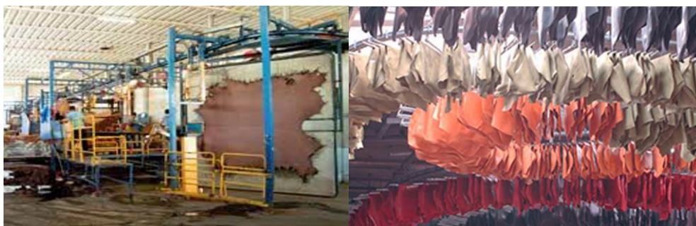
Chart 5 – Frame drying and Overhead chain drying
