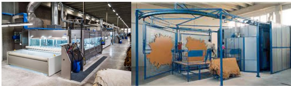
Chart 6 – Spraying Machine and Dry Nailing finishing techniques
