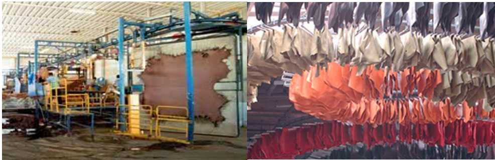
Chart 5 – Frame drying and Overhead chain drying
